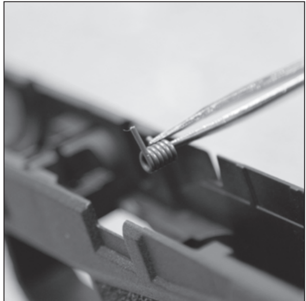
Figure 68 — Placing the magazine catch spring inside the magazine catch slot
