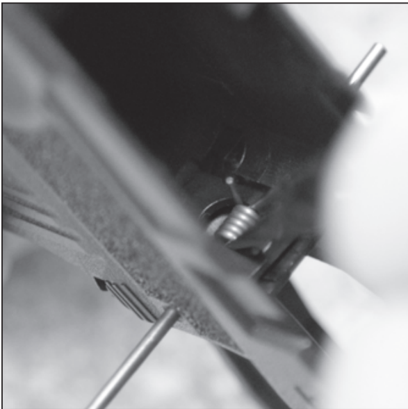
Figure 69 — Insert the punch through the spring to hold it in place
