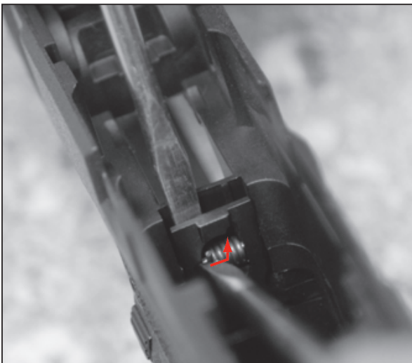
Figure 71 — Pushing the magazine catch spring into position through a notch in the magazine catch
